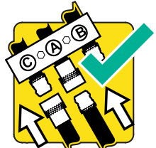
4. ENSURE HYDRAULIC HOSES ARE CLEAN AND ATTACHED
