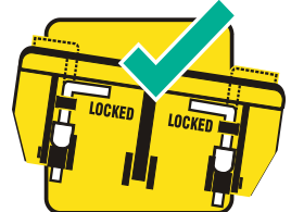
3. ENSURE BOTH (2) ATTACHMENT LOCK PINS ARE FULLY ENGAGED
